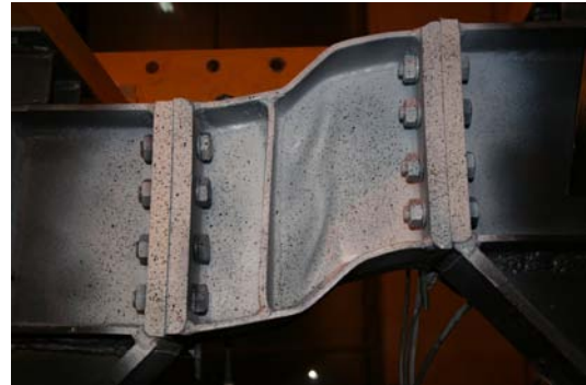
Failure mode of specimen L20m1
