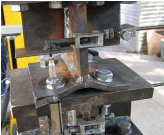
Failure mode of a T-stub specimen by end-plate bending
