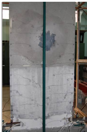
General view of testing frame and distribution of cracks during testing
