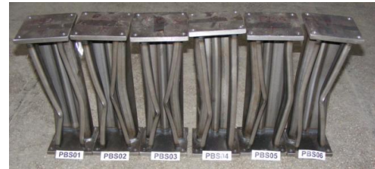
Tested stub columns – brut section P95x2.6
