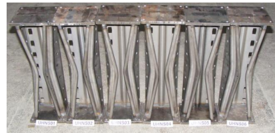
Tested stub columns – net section UH125x3.2
