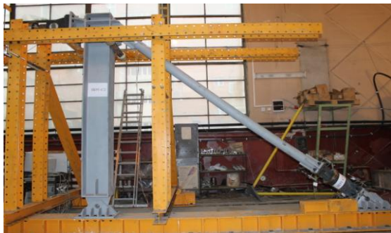
Experimental testing of a brace with a damper device
