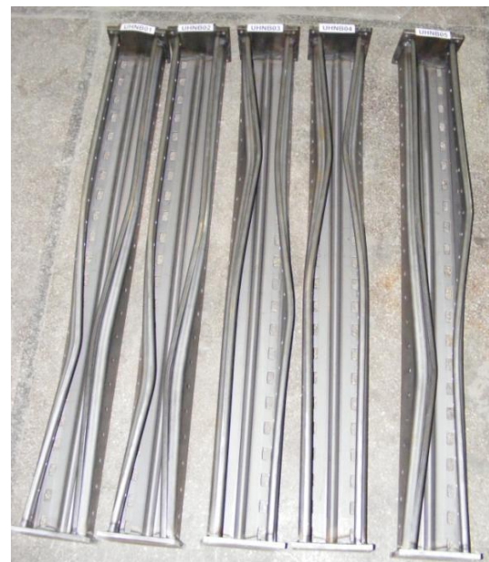
Tested columns – net section UH125x3.2 – distortional buckling
