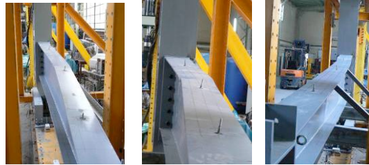
Failure of the specimen with 8 mm tapered web
