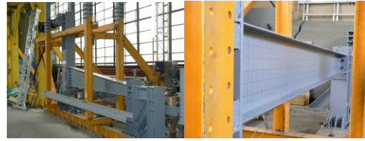
Test arrangement for beam-column tests
