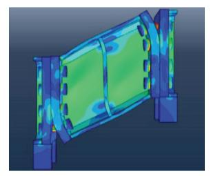
Once all links from a story are removed, all structural components from that story are in elastic range of response.
