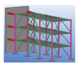
•A solution that uses temporary braces with viscous dampers mounted on the structure during link removal was analysed and chosen in order that the link removal process to be a safe one;
