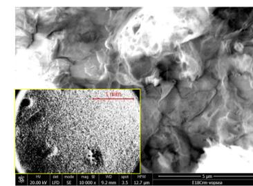
Fig 18. SEM micrographs of the coating prepared with pigment B.
