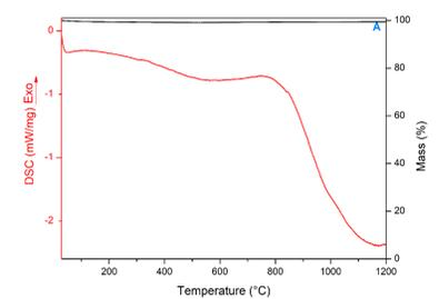
Fig 7. TG-DSC curves of the as-obtained pigment A.
