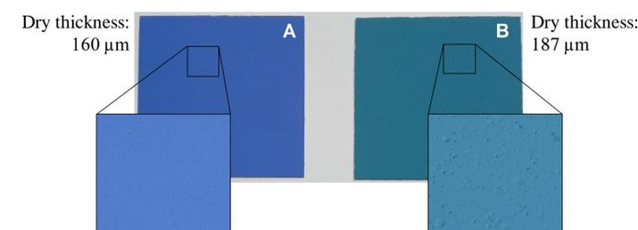
Fig 16. Coatings prepared with pigments A and B.
