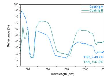
Fig 19. DRS of the coatings prepared with pigments A and B.
