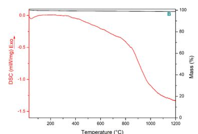
Fig 12. TG-DSC curves of the as-obtained pigment B.
