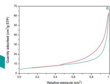
Fig 11. Adsorption-desorption isotherm of pigment B.
