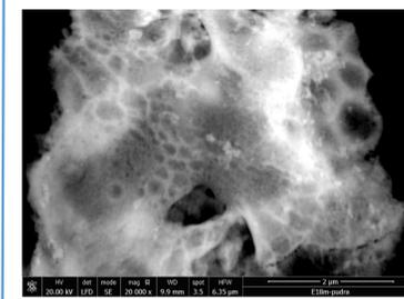
Fig 17. SEM micrograph of the coating prepared with pigment A.
