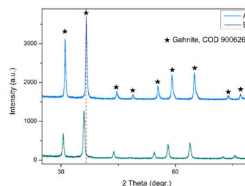
Fig 8. XRD patterns of pigments A and B.
