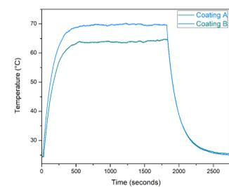
Fig 20. Temperature variation of the coatings prepared with pigments A and B, during IR irradiation.
