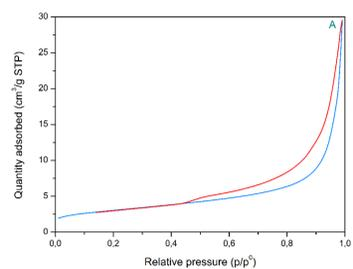
Fig 6. Adsorption-desorption isotherm of pigment A.
