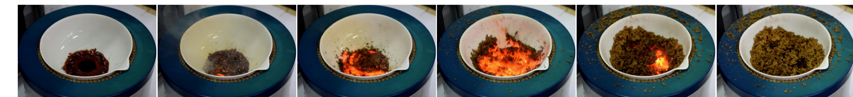
Fig. 1. Still images captured during the evolution of a typical combustion reaction ( x = 0.75 , sample LAF 0.75).
