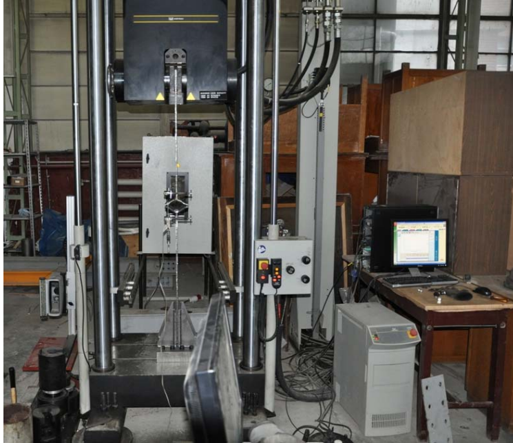
Figure 45. Test set up with the universal machine for room temperature tests
