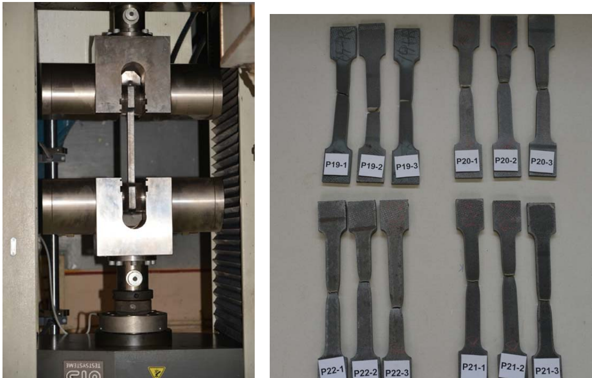
Figure 40. Coupon specimen in universal machine (left) and failure mode (right)
