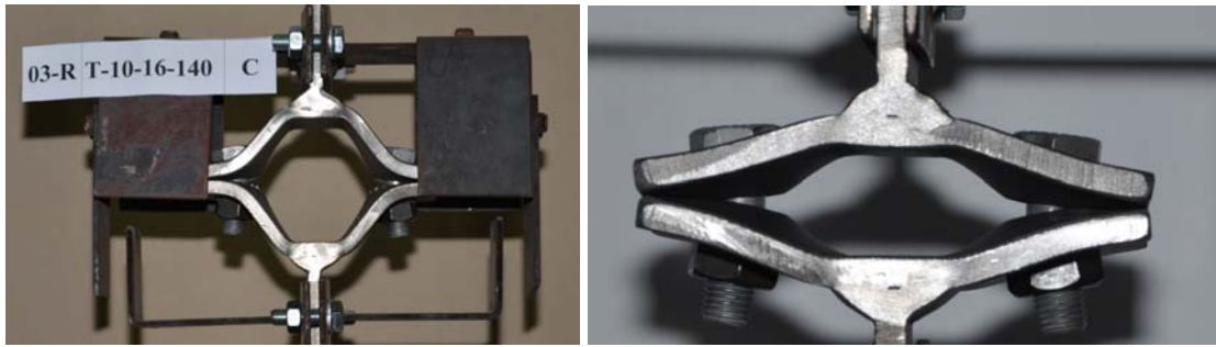
Figure 56. Failure mode 1 (left, T-10-16-140) and failure mode 2 (right, T-10-16-100)
