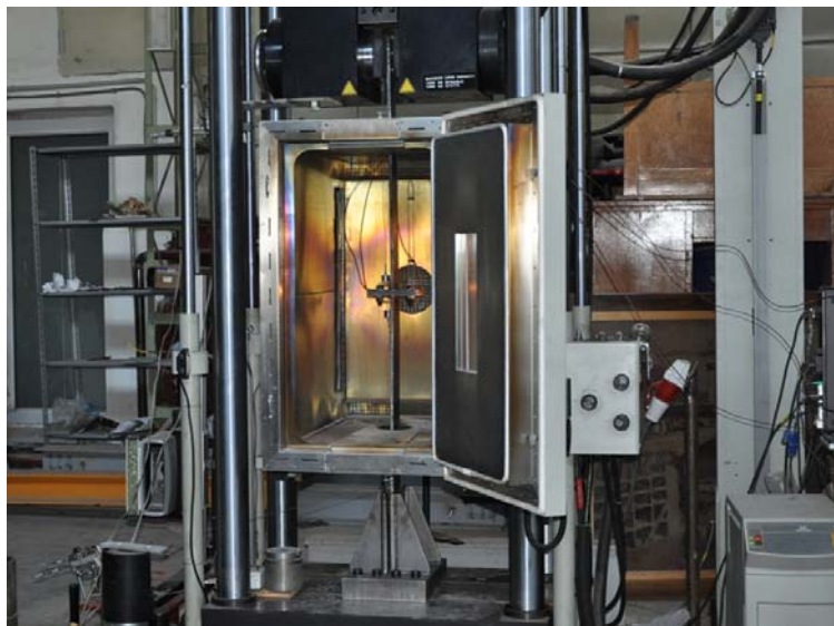
Figure 46. Test set up with the furnace for elevated temperature
