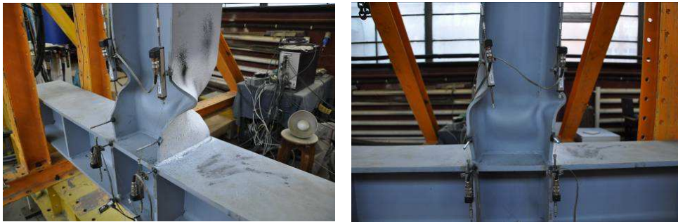
Figure 37. Failure of DB-C RLD specimen through plastic hinges in RBS
