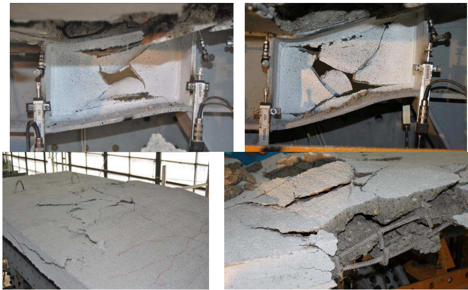
Figure 73. Damage of the fixed link and concrete slab for EBF_LF_Comp1 (left) and Comp2 (right) specimens.
