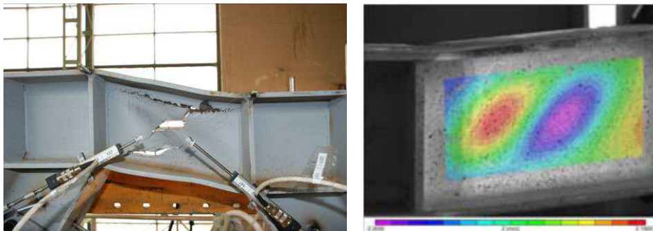
Figure 69. Shear failure of EBF_M_LF-C specimen
