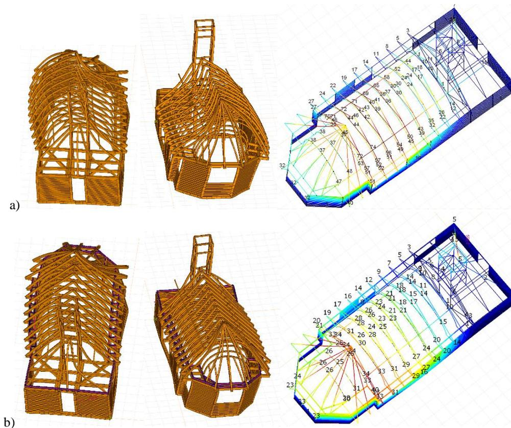
**Fig. 6.16** Deformed shape of the church: a) before and b) after consolidation
