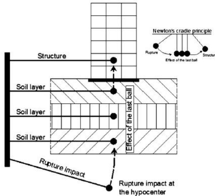
Fig. 3.40 Soil-Structure interaction and the analogy with Newton's cradle
