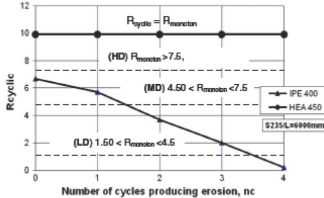
Fig. 3.32 Influence of the cross-section conformation on the cyclic ductility
