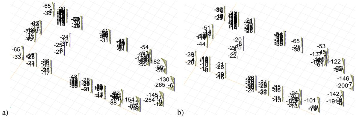
**Fig. 6.19** Maximum values of compression stress in columns: a) before and b) after consolidation
