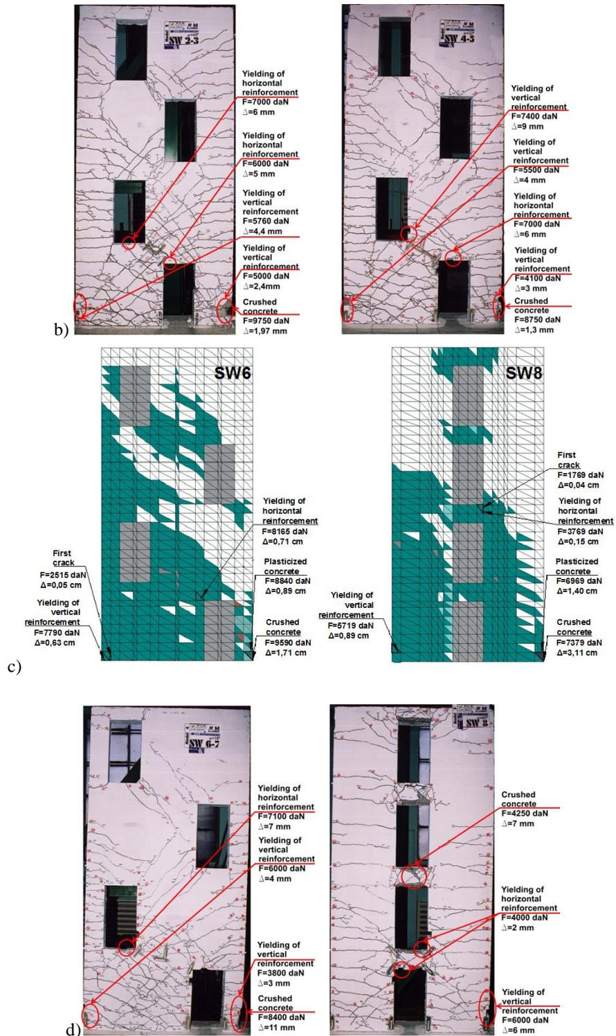
**Fig. 2.7** a,b) Theoretical and experimental failure modes of shear walls SW2-3 and SW4-5
