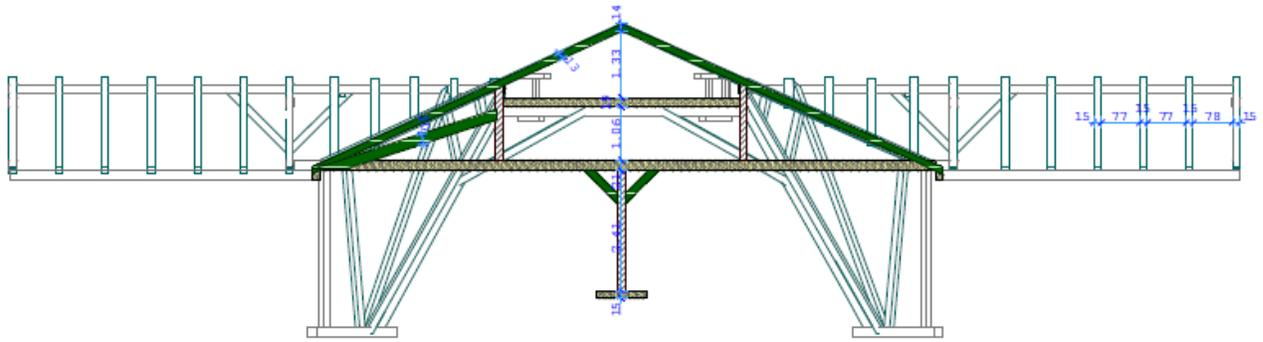
**Fig. 6.25** a) Arrangement plan of the roof framing elements b) Transversal roof framing section
