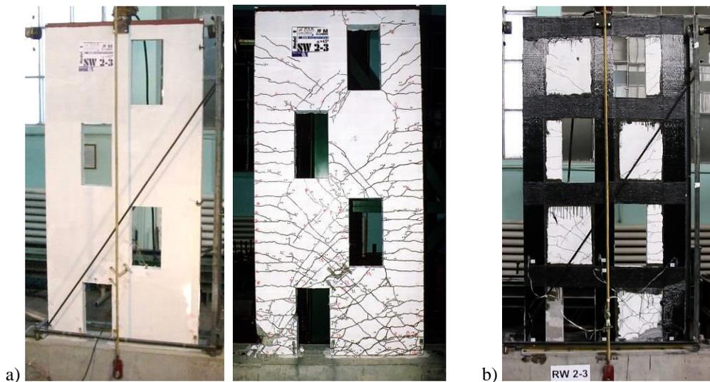
**Fig. 2.11** Test models a) before and after testing (SW23); b) after consolidation (RW23)
