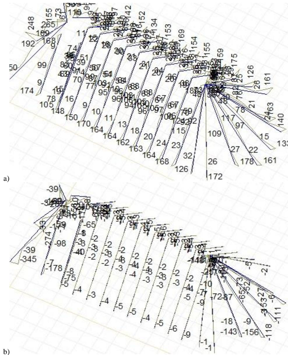
**Fig. 6.21** Maximum values of stress in rafters: a) before and b) after consolidation
