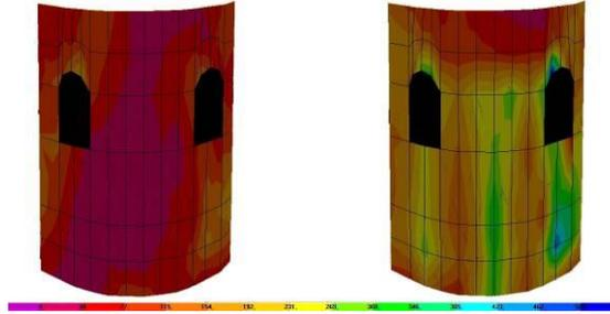
Fig. 5.11 Shear stress diagram S12 for East wall
