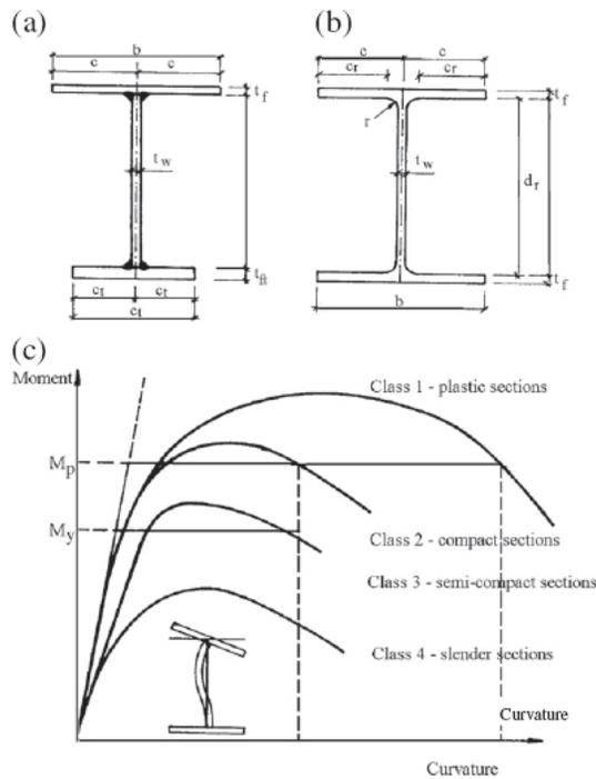
Fig. 3.22 Cross-section classification according to current design codes (i.e. Eurocode 3)
