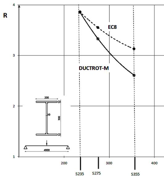
**Fig. 3.13** Influence of yield stress and steel grade on rotation capacity
