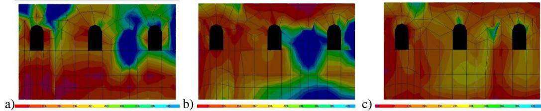
**Fig. 5.9** Stress diagram for North wall a) Tension stress S11; b) Compression stress S22 c) Shear stress S12
