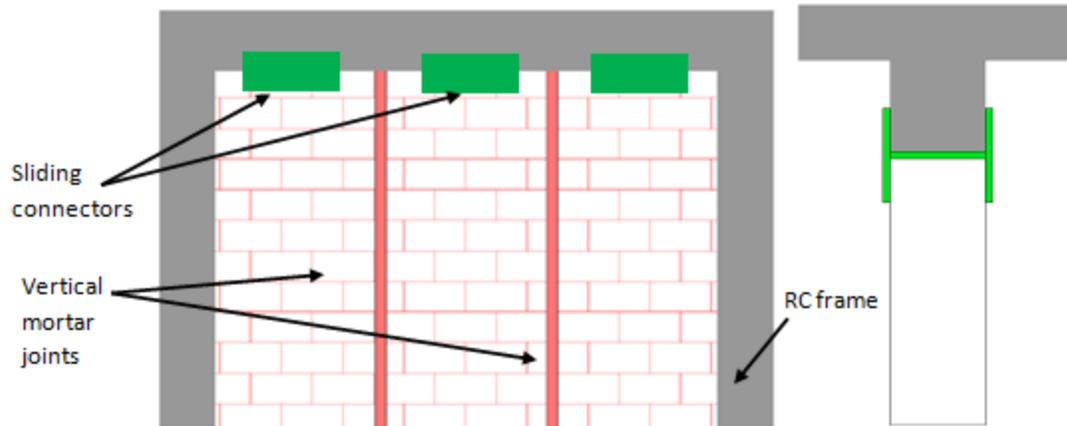
**Fig. 2.59** Infill masonry walls divided by vertical mortar joints and sliding connectors
