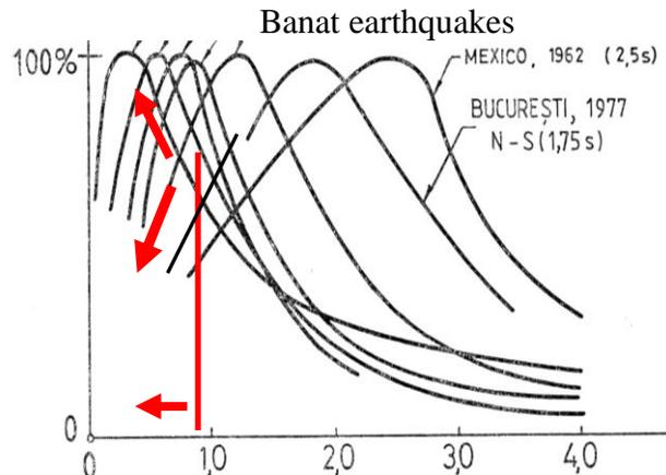
Fig. 5.14 Effects of rigidity increasing by strengthening
