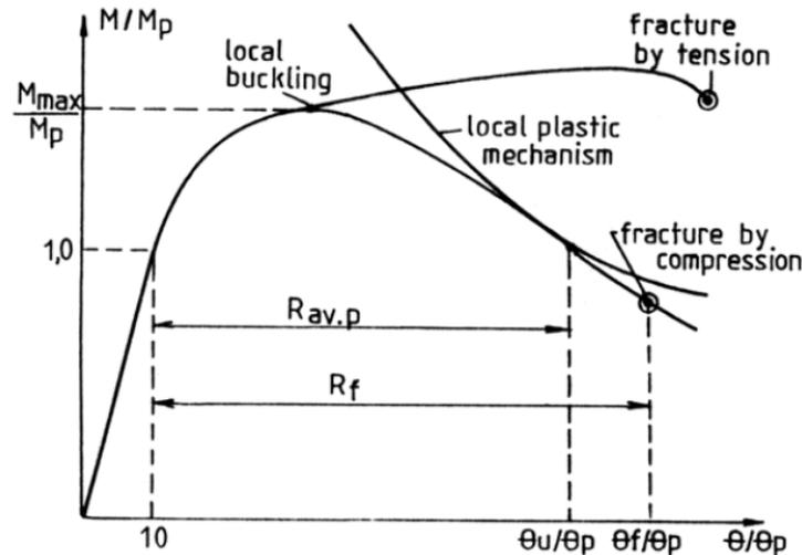
Fig. 3.7 Definition of the rotation capacity of a steel member
