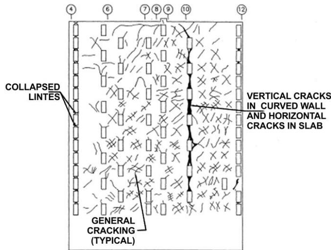
**Fig. 2.3** Brittle failures of coupled beams at the shear wall with staggered openings from Hanga-Roa building, Chile, 1985 [2.22]
