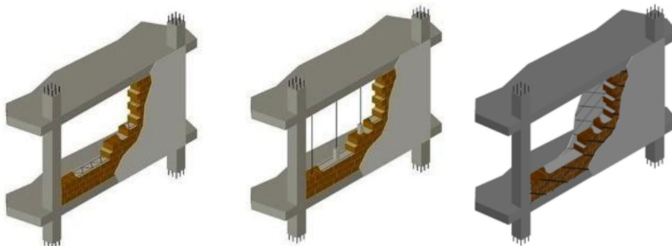
**Fig. 2.53** Solutions: horizontal reinforcement; horizontal and vertical reinforcement; new types of plastered wire meshes (from left to right)
