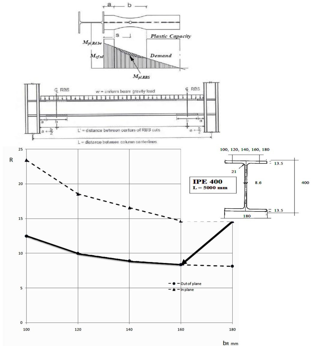
Fig. 11 Rotation capacity for RBS
