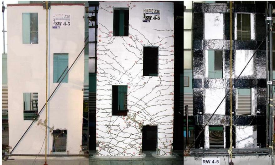
**Fig. 2.13** Test models a) before and after testing (SW45); b) after consolidation (RW45)
