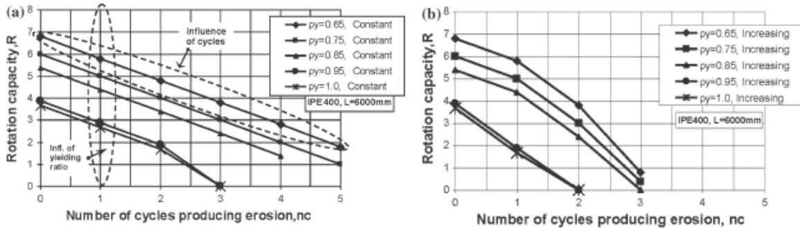
Fig. 3.35 Influence of the yielding ratio on the cyclic rotation capacity
