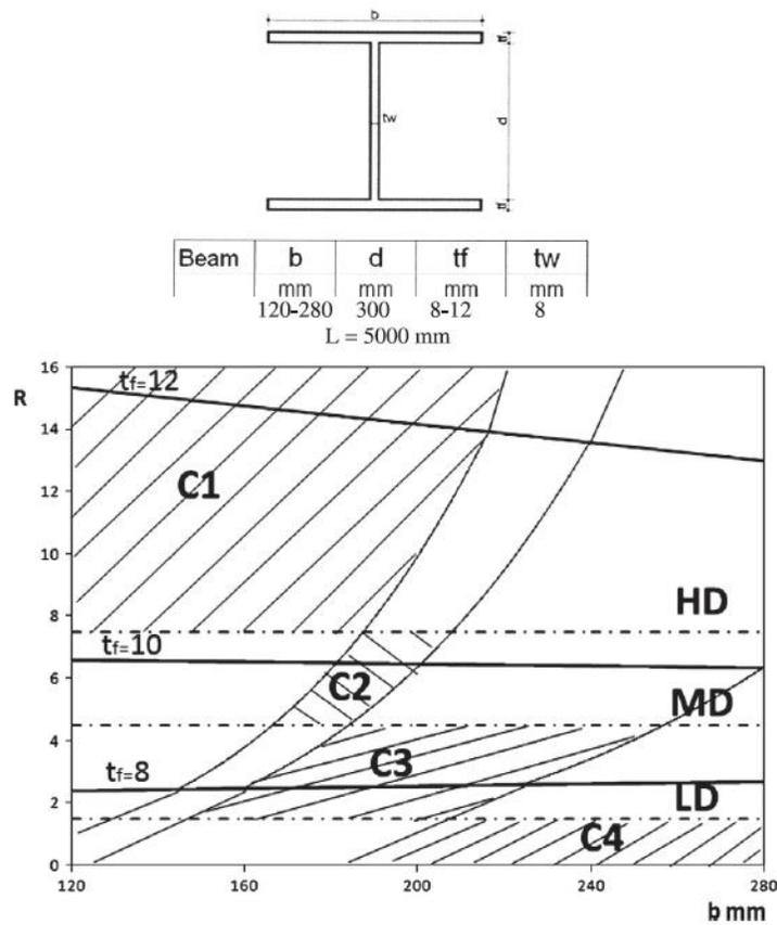
**Fig. 3.24** Member ductility vs. cross section ductility for a profile with C1 class for the web
