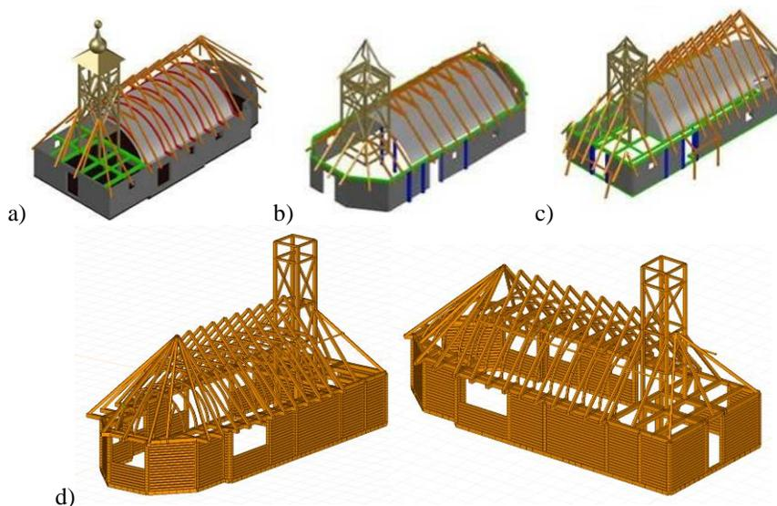
**Fig. 6.6** Bearing structure 3D model of churches a) Curtea, b) Crivina de Sus, c) Romanesti, d) Dobresti
