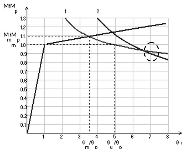
Fig. 3.6 Interaction between in-plane and out-of-plane local plastic mechanisms
