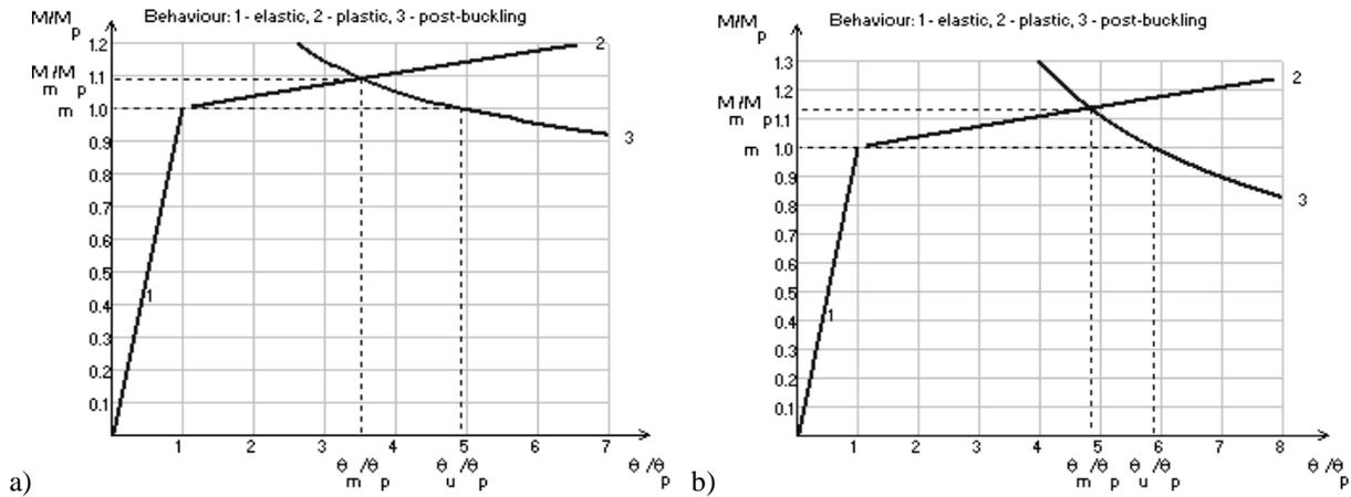
Fig. 3.5 M- $\theta$  a) for in plane plastic mechanism, b) for out of plane plastic mechanism
