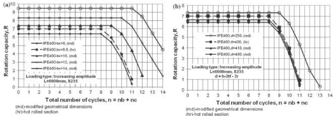
Fig. 3.33 Influence of the web slenderness (height vs. thickness) on the cyclic ductility
