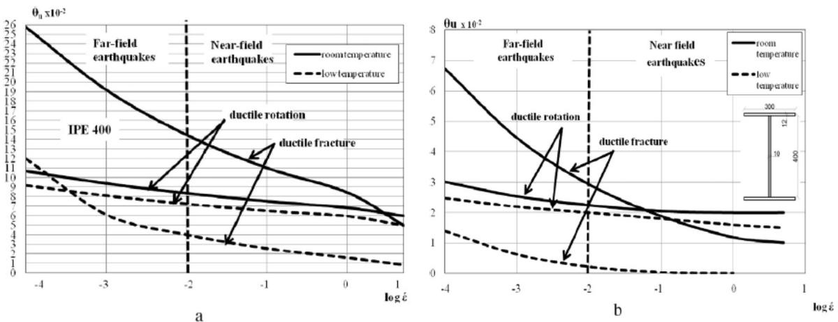
Fig. 3.42 Influence of strain rate on the ultimate rotation capacity
