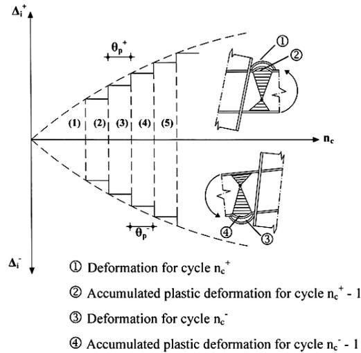
**Fig. 3.27** Plastic collapse mechanism at the member level
