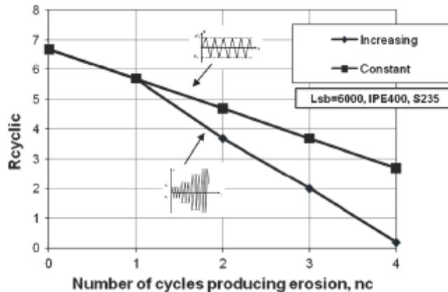
Fig. 3.31 Influence of the loading type on the cyclic ductility
