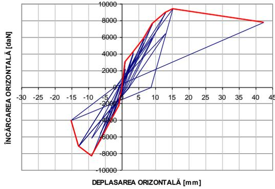
a) Force-displacement diagram of SW8
