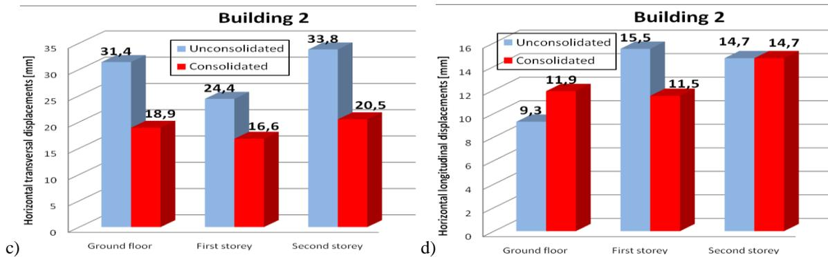
**Fig. 5.28** Maximum comparative values of horizontal displacements on transversal and longitudinal directions before and after strengthening of the buildings, a- b) building 1, c-d) building 2
