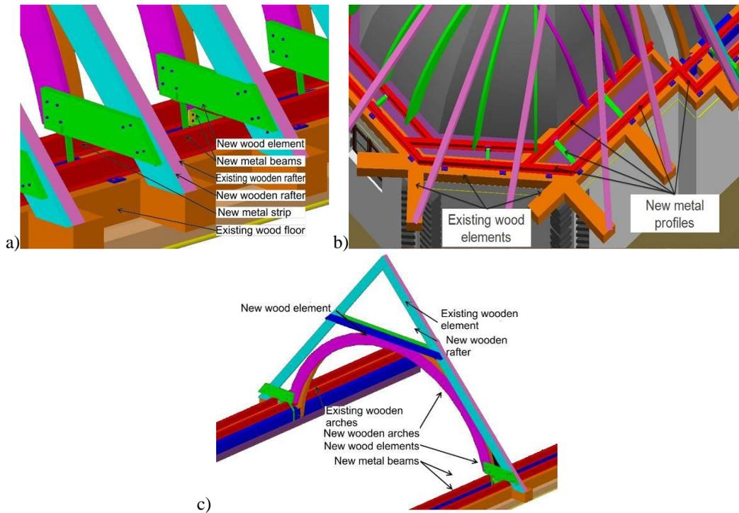
**Fig. 6.14** a), b), c) Consolidation solutions for beams and arches from nave and altar
