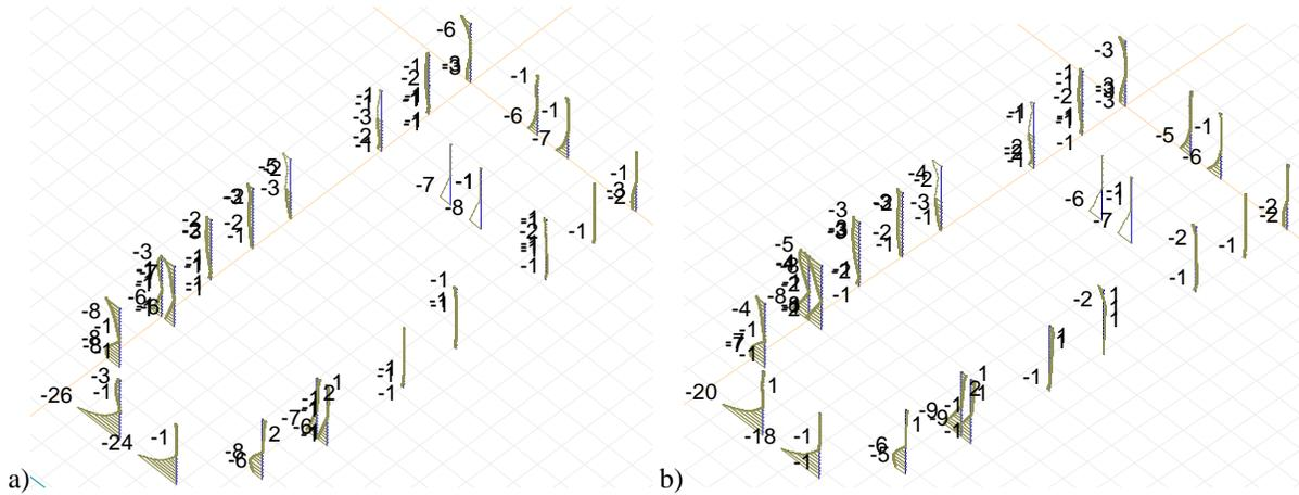
**Fig. 6.18** Maximum values of bending moments  $M$  in columns: a) before and b) after consolidation
