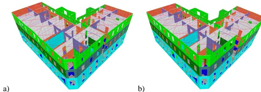
**Fig. 5.25** The vibration modes 1 and 2 of the consolidated building
