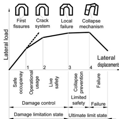
**Fig. 5.1** Behaviour of a masonry triumphal arch [5.5]
