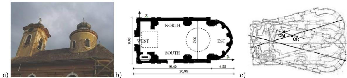
**Fig. 5.5** a) view of the towers; b) horizontal section; c) position of centre of mass and rigidity
