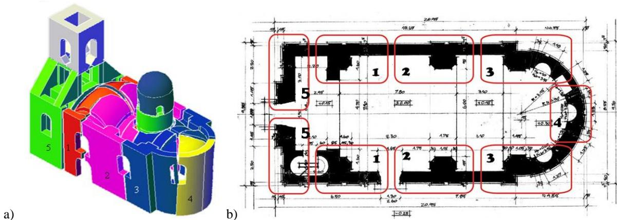
Fig. 5.12 a) blocks system in ultimate limit state; b) in plan dimensions and positions of blocks
