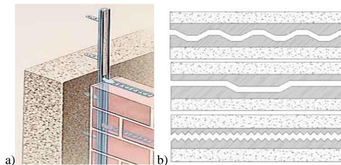
**Fig. 2.60** a) Reinforcement connection; b) various sliding joints configurations
