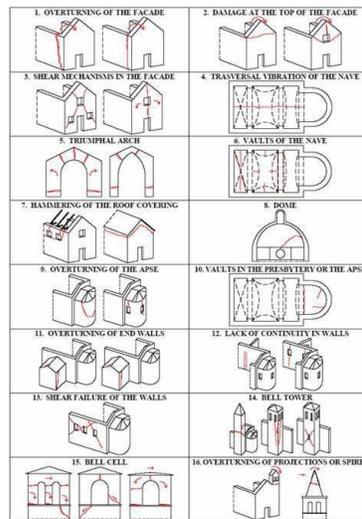
**Fig. 5.2** Behaviour of a masonry Romanesque church. Masonry rigid block [5.10]
