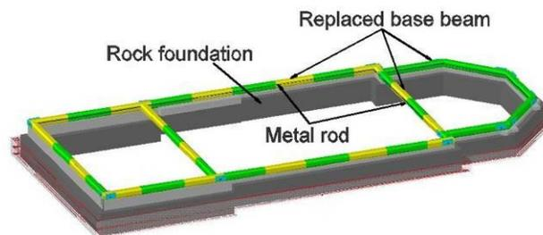
**Fig. 6.12** The consolidation solution of the foundation and of the base beam of the church
