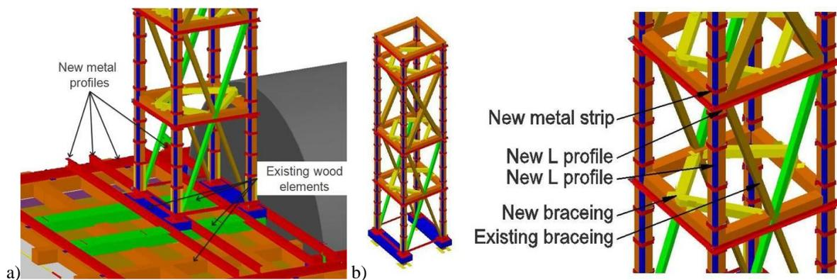
**Fig. 6.15** a), b) Consolidation solutions for the wooden columns and beams of the tower of the church
