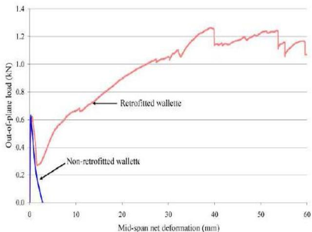
**Fig. 7.4** Failure patterns of brick masonry wallets with and without retrofitting by PPB mesh and the out-of-plane load variation [7.5]
