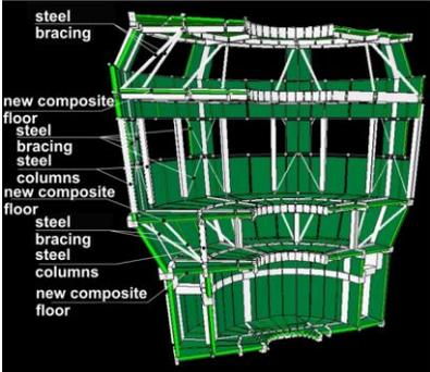
Fig. 4.6 Consolidation solution 2
