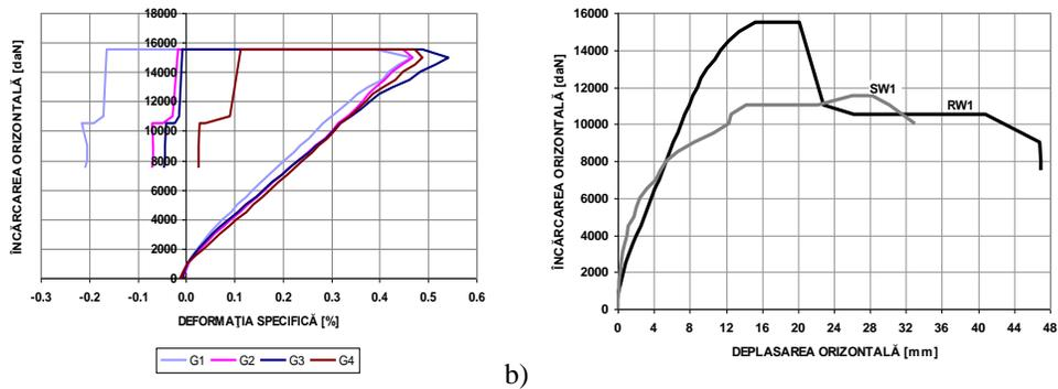
**Fig. 2.10** a) Strains in the composite material; b) Force-displacement diagrams of models SW1 and RW1
