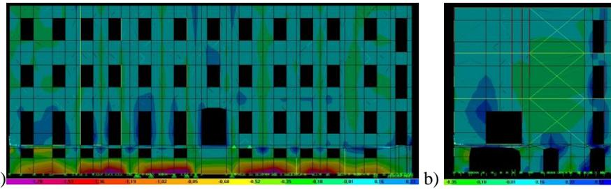
Fig. 5.26 Normal stresses in a) external longitudinal wall - axis A; b) internal transversal wall – axis 5
