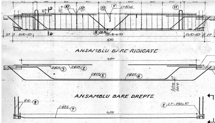
Fig. 2.20 RC precast beam
