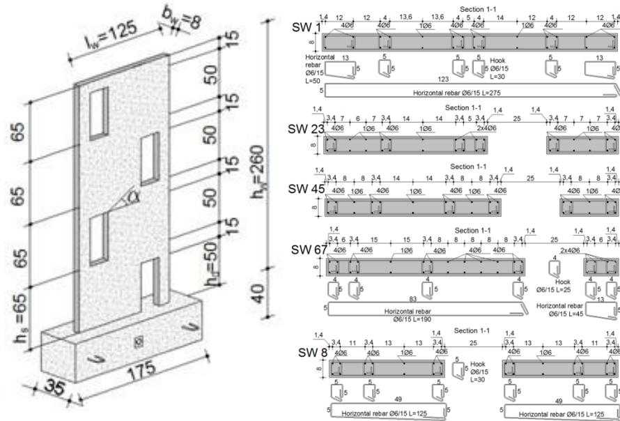
Fig. 2.4 Geometry and reinforcement layout of the test models
