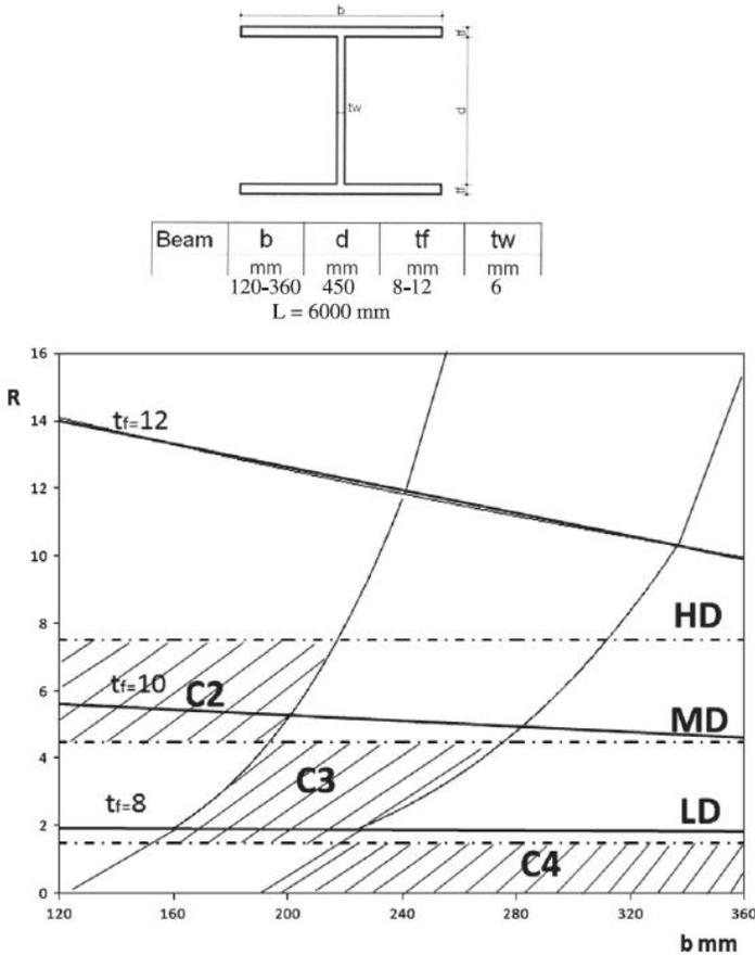
Fig. 3.25 Member ductility vs. cross section ductility for a profile with C2 class for the web
