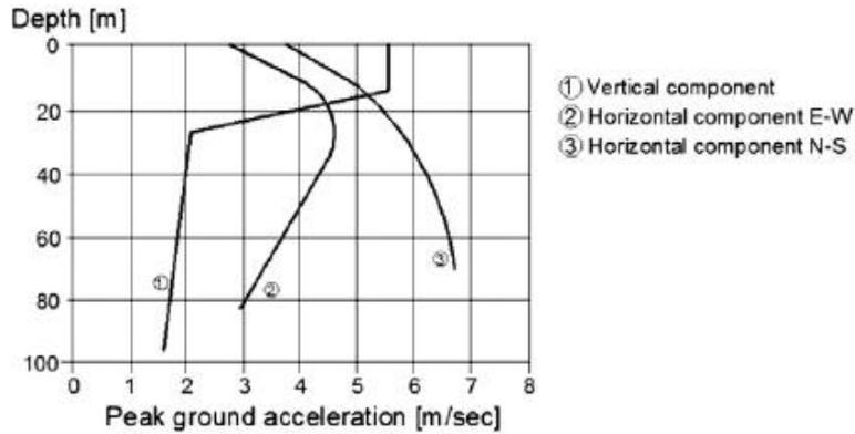
Fig. 3.41 Measured acceleration on free site [3.22], [3.23]
