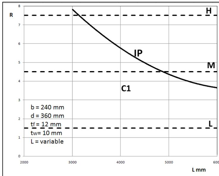
**Fig. 3.19** Influence of beam span
