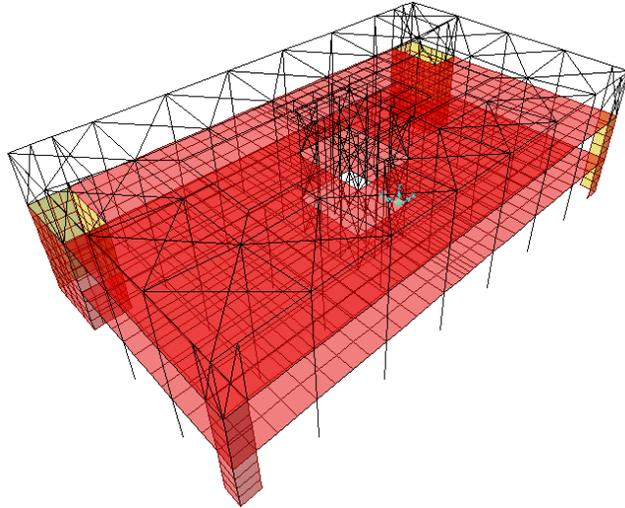
**Fig. 2.25** Discretization of structure
