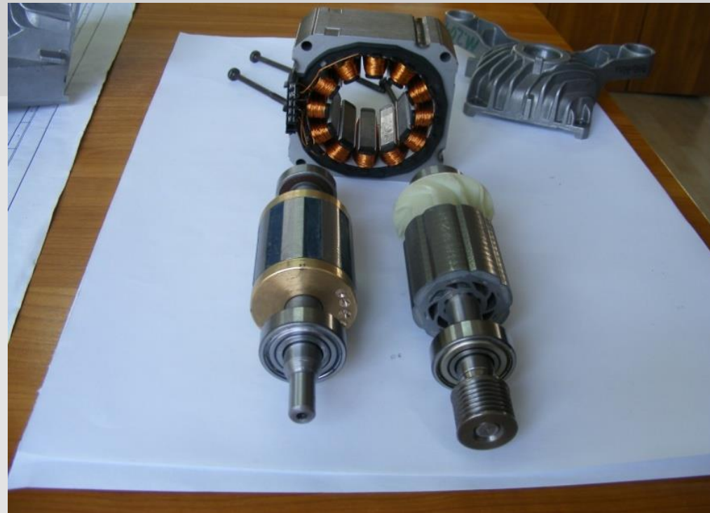
PMSM with flux concentrator rotor PMSM-FC.
