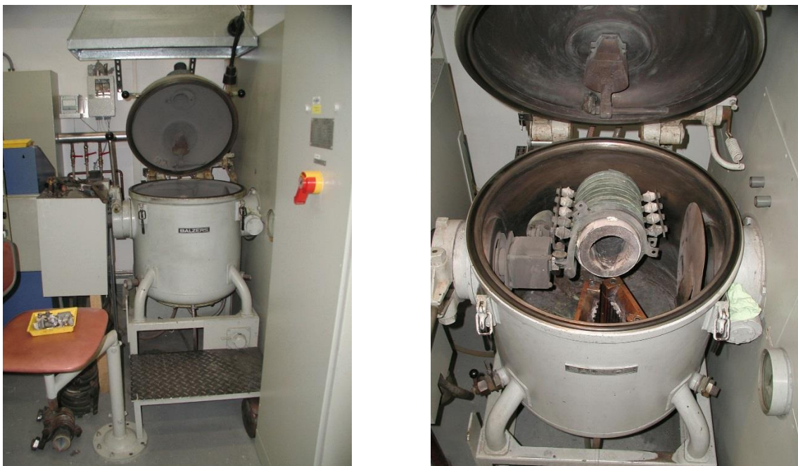
Fig. 3.1 Induction melting furnace used in the current work. Left: general view. Right: details where the coil, the melting crucible and the mold can be seen.
