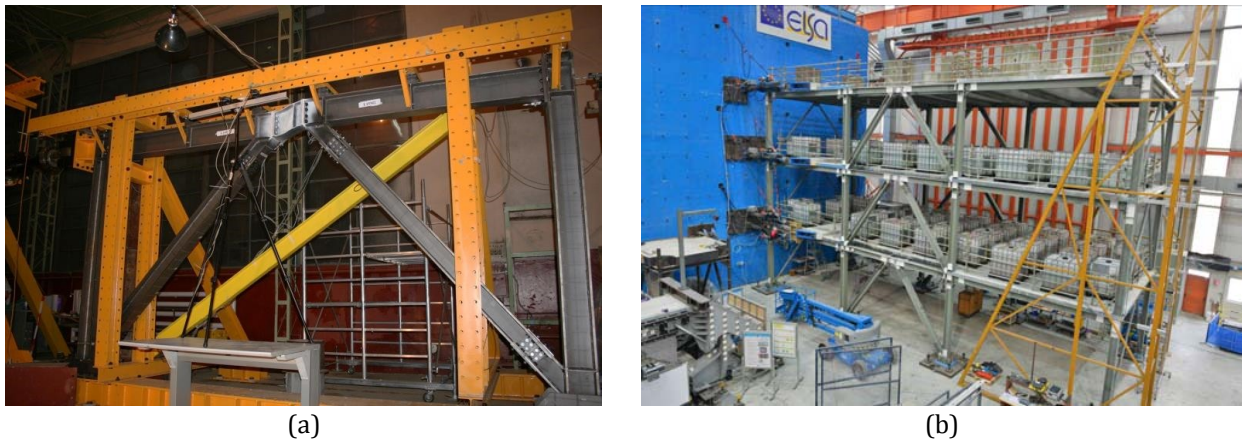
Figure 1. Experimental test on almost full-scale frame with bolted links in the Structural Laboratory of the Politehnica University of Timisoara, CEMSIG research centre (a) and the experimental mock-up in front of the reaction wall of the European Laboratory for Structural Assessment (ELSA) at JRC in Ispra (b).
