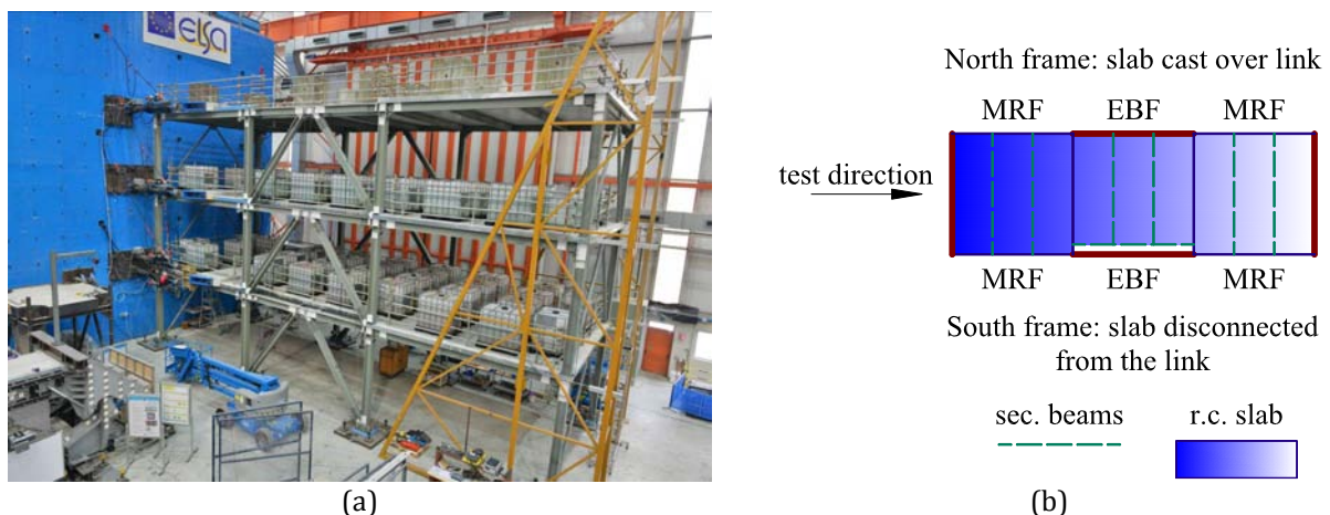
Figure 27. The experimental mock-up in front of the reaction wall (a) and plan layout (b) of the test structure.
