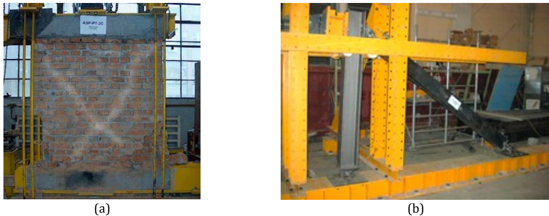
Figure 4. Testing of a masonry wall (a) and a buckling restrained brace (b).
