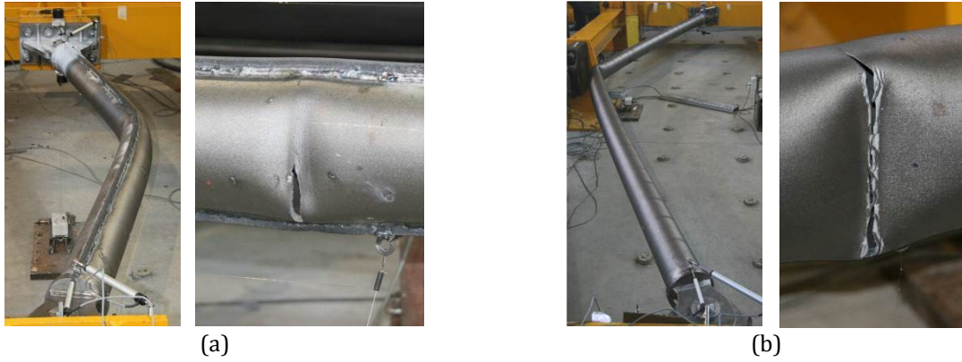
Figure 134. Failure mode of the SP27-2 (a) and SP59-1 (b) specimens.
