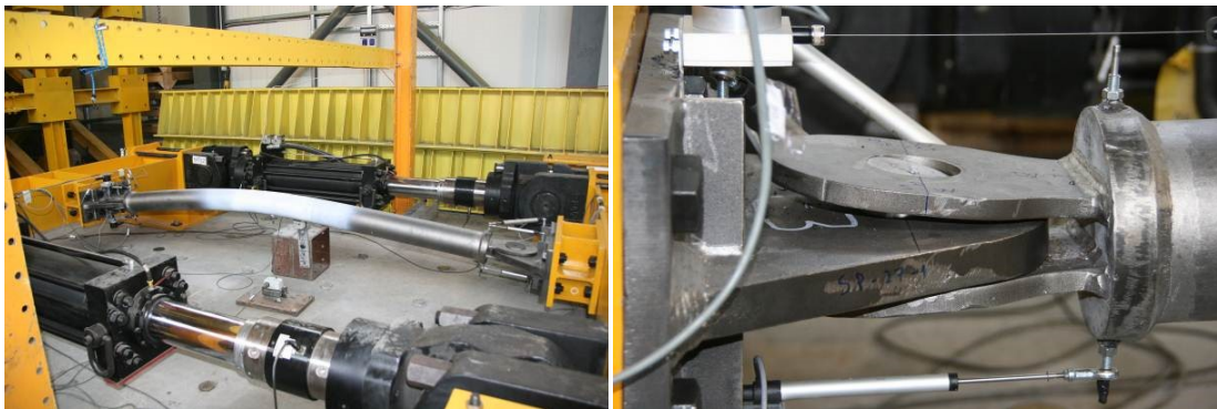
Figure 133. Failure mode of the SP27-1 specimen.
