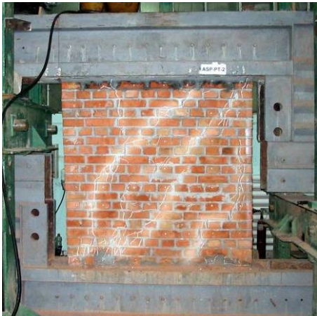
Figure 121. Failure mode for ASP-PT-2m
