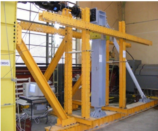
Figure 140 Experimental test setup for brace tests
