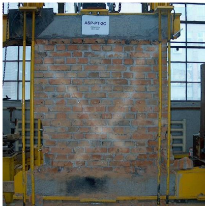
Figure 123. Failure mode for ASP-PT-2C
