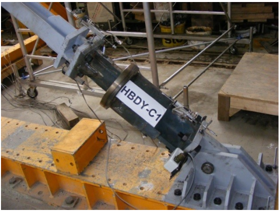
Figure 141 Experimental test setup for brace with damper assembly tests
