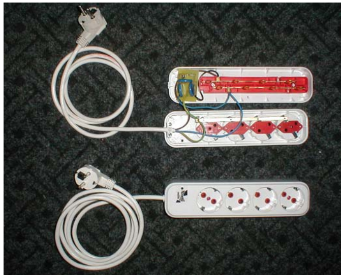
Fig. C4. Multi-plug block protected against overvoltages – BMS01
