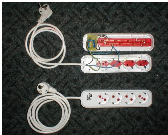
Fig. 2.10.3. Multi-plug Block Protected from Overvoltage – BMS-01
