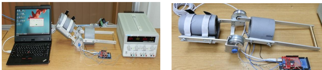
Fig. 3.1.15. The elbow module with two brakes and angular sensor
