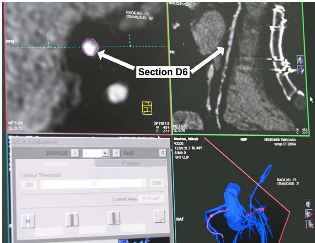
Figure 2.1: Physiologically realistic geometry measurements using CT image techniques. Area measurements of the different stenosed section. For position of section D6 see Figure 3.2.
