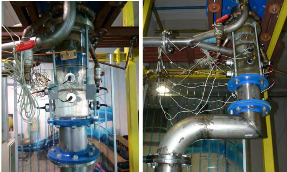
Figure ii.2.34 Photos of the test section with two geometrical configurations: straight (S) and 90° heel elbow together with pipe length extensions of 0.2 m (HE90E02).
