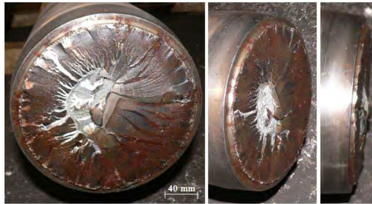
Figure ii.3.6. Fracture surface of the pump storage shaft: frontal view, low angle view and lateral view.
