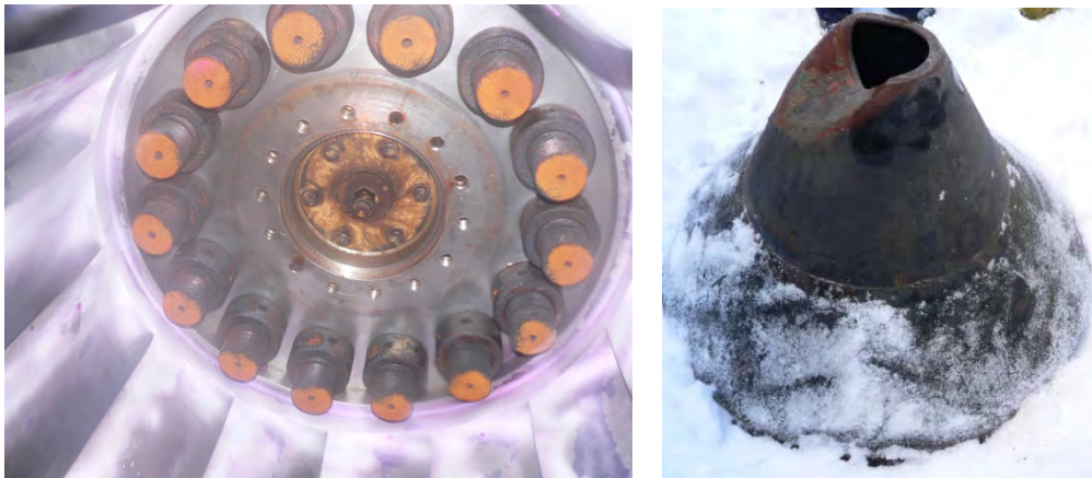
Figure ii.1.5 The runner cone was removed due to the vortex rope generated at part load conditions. The view of the runner without cone ogive and the runner cone ogive recovered from draft tube.
