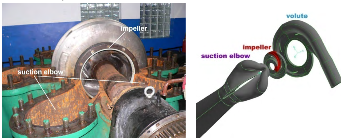
Figure ii.3.7. The hydraulic passage of the investigated storage pump and 3D computational domains. The three-dimensional complex geometry of the suction elbow and the mesh with 465635 cells are plotted in Figure ii.3.8. The mesh is refined near to outlet surface in order to capture the non-uniform distribution of the
