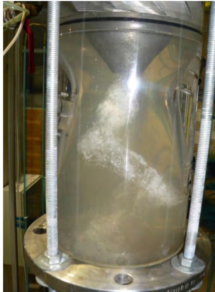
Figure ii.2.7 The visualization of the cavitating vortex rope from the cone of the test section.
