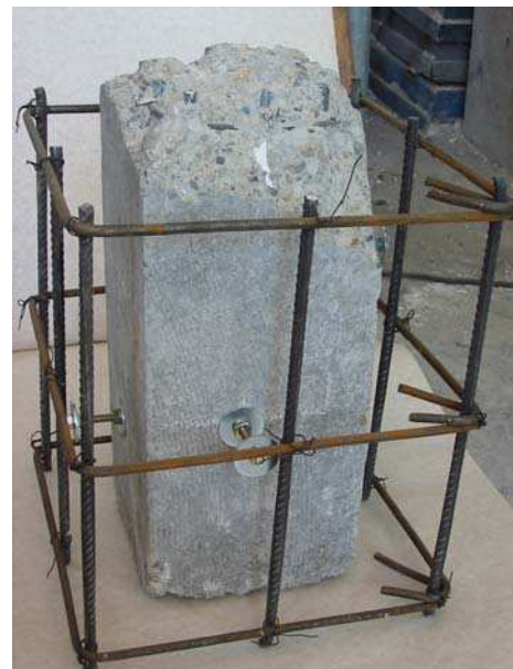
Fig. 4. Using of mechanical anchored connectors.
