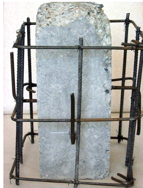
Fig. 3. Using of chemical anchored connectors.
