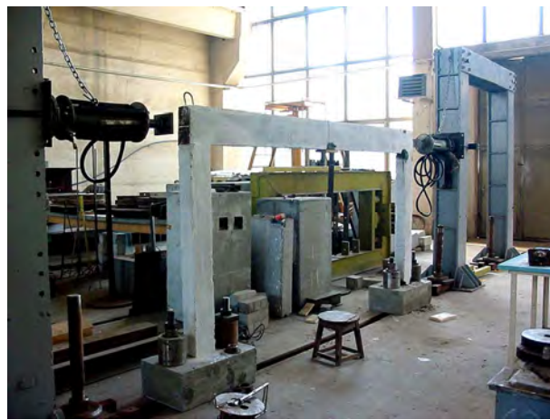
Figure 2.10. Reinforced concrete frame model
