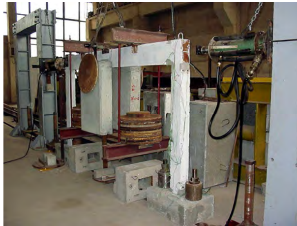
Figure 2.15. RC frame – experimental loading
