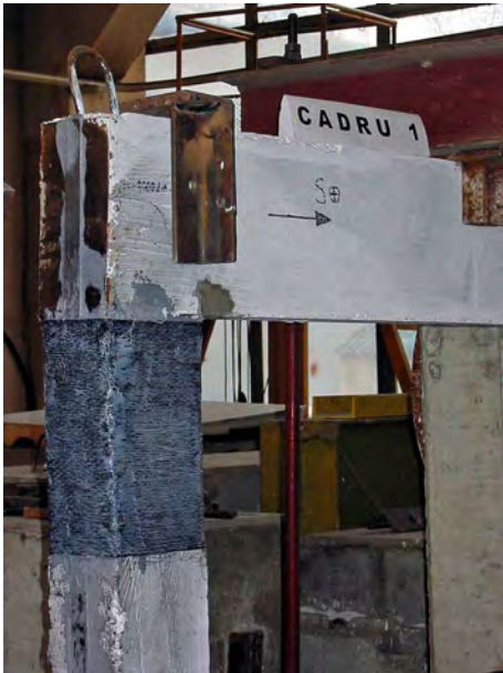
Figure 2.18. Glued anchorage – Frame 1 (CADRU 1)
