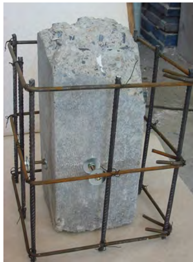
Figure 2.5. Using of mechanical anchored connectors
