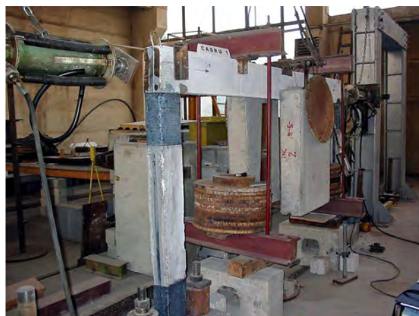
Figure 2.17. RC frame + CFRP strengthening
