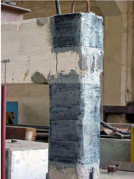
Figure 2.19. Wrap anchorage – Frame 2 (CADRU 2)
