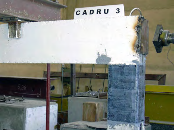
Figure 2.20. Mechanical anchorage – Frame 3 (CADRU 3)
