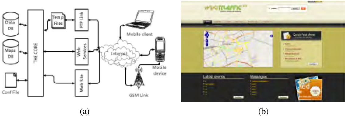
Figure 4.2: System architecture (a) and web application interface (b) [49].
