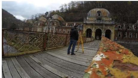
Fig 9. Scanning the facade and the bridge of iron Herculane
