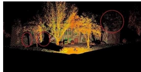
Fig 5. Limitations of TLS capture in areas with dense vegetation
