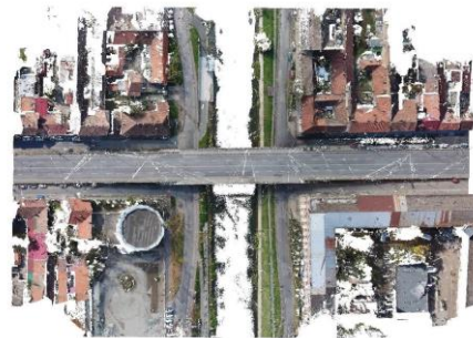
Fig 13. Point cloud extracted from captured images (Cuzic O.Ș. 2022)
