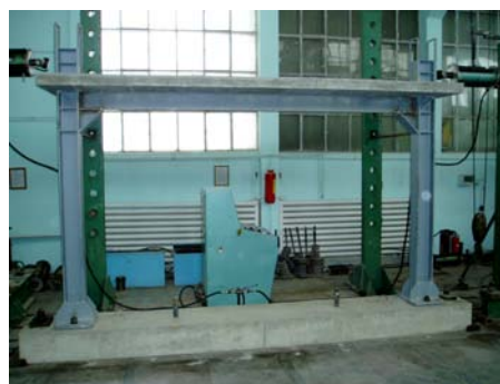
Experimental frames tested at horizontal loads
