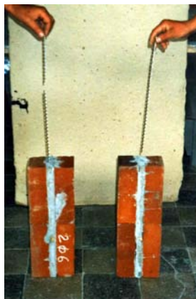
Brutt Helical Bars failure
