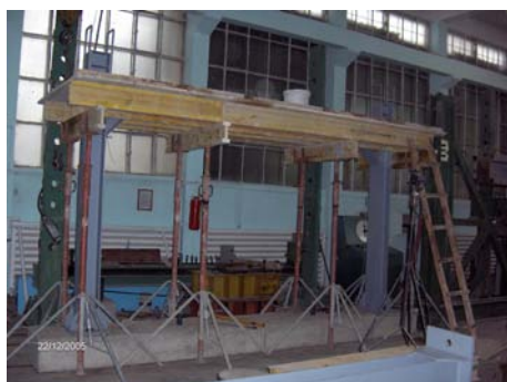
Experimental composite steel-concrete frames
