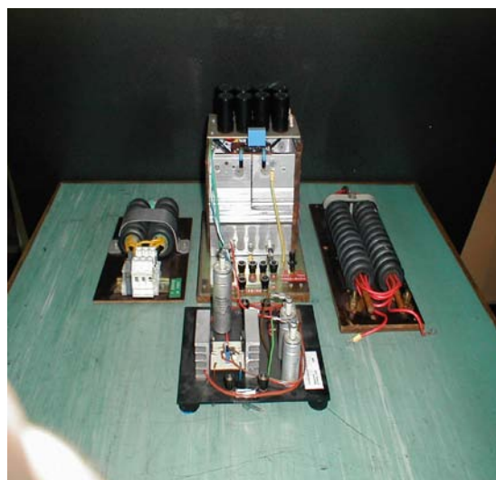
High frequency welding transformers.
