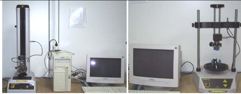
Multi Test 5-i Computer-controlled system. Vortex (-i) Computer-controlled torque system
