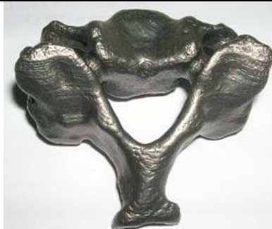
Titanium vertebra realized on Arcam S12 machine
