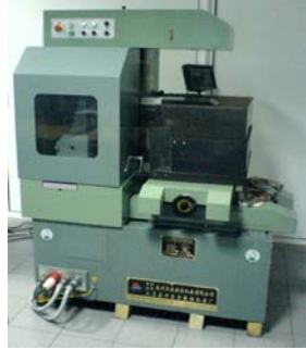
Maxillo-facial plate implant fabrication on white EDM machine
