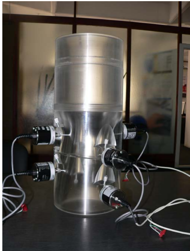
Test section for pressure measurements
