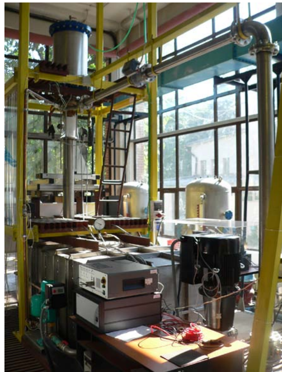
Closed loop test rig for experimental investigations of swirling flows and laser system to measure the velocity profiles
