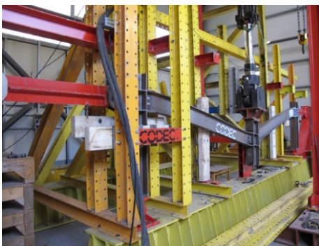
Fig. 1a. Joint specimen after the test
